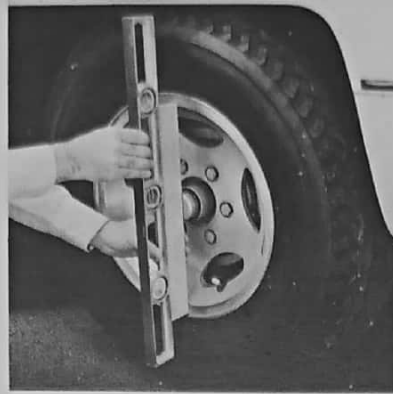
Camber Adjustment Check
