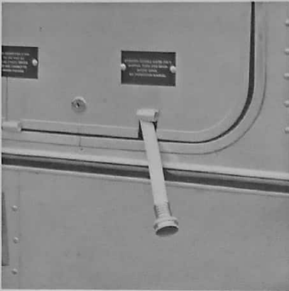
City Water Connection
