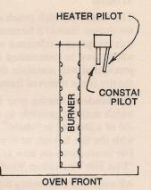
the dial. This will allow gas to flow to the heater Pilot Tube, to be ignited by the Constant Pilot.
